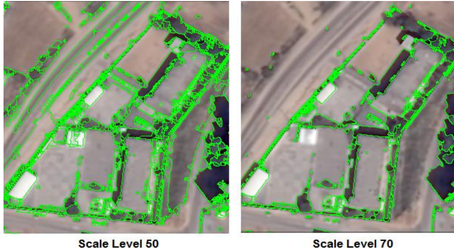
Figure 3-12: Image segmentation result at different levels
